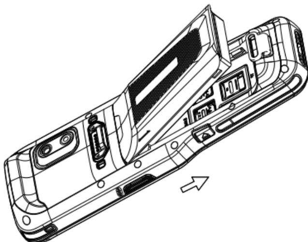
\* Please peel off the yellow insulation sticker pasted on the positive and negative of battery before turning on the device
