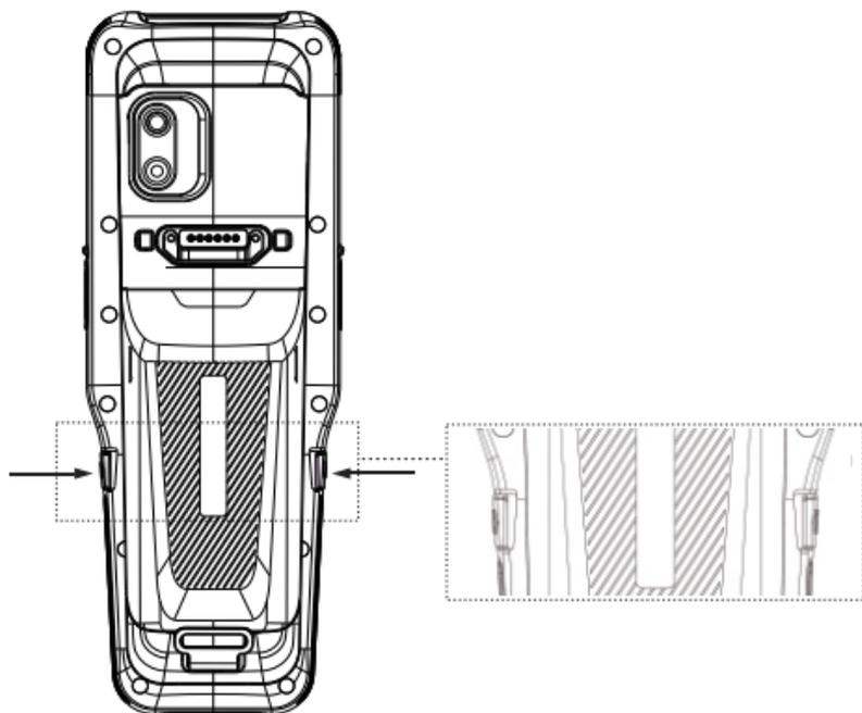
2. Press the switch on both sides and the battery will fall down naturally.
