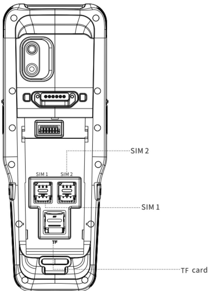
(Note: The device only supports NANO SIM card)
